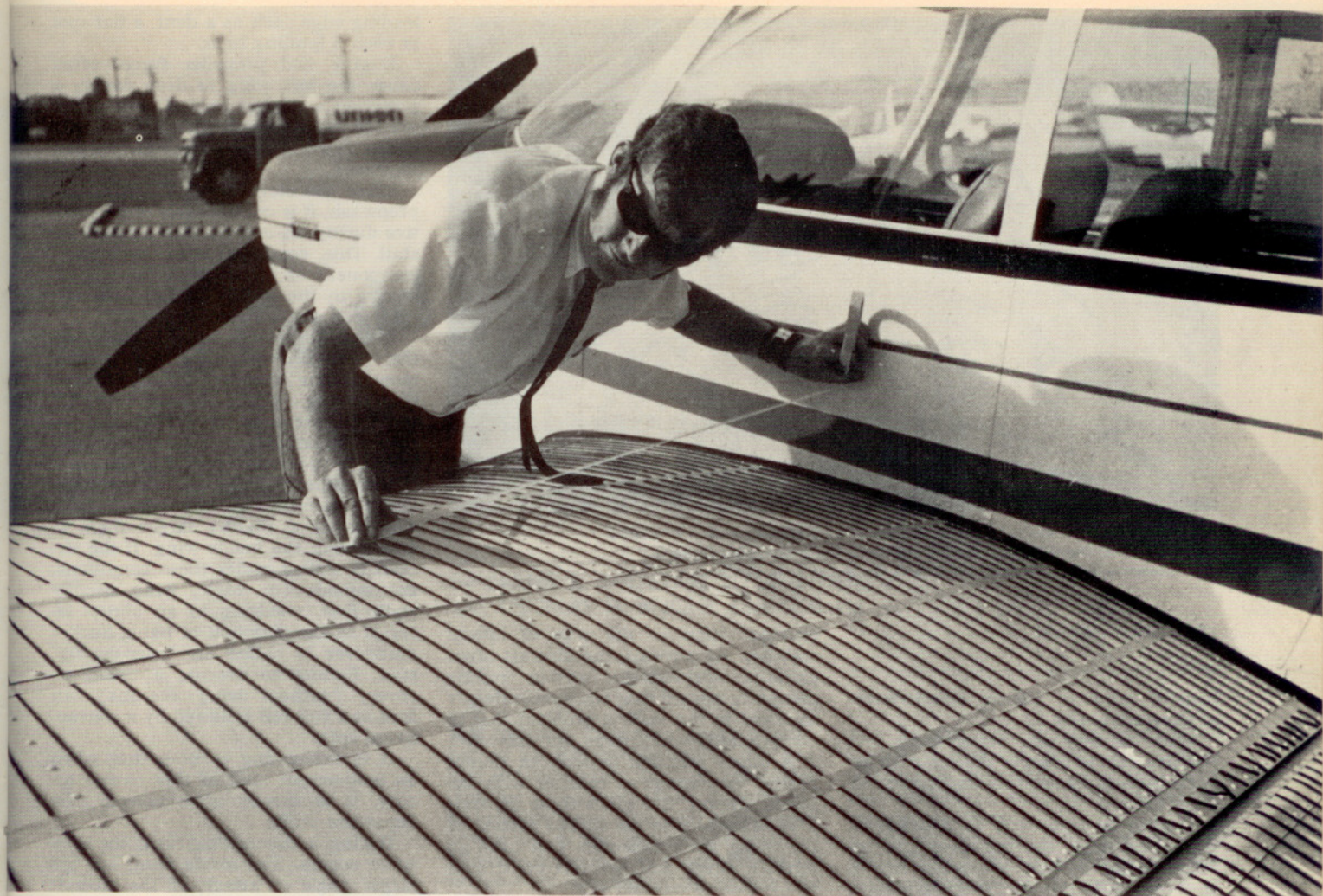
Cal Pitts applies masking tape over yarn wrapped around Cherokee 180 wing. Strands were then snipped with scissors to form free-flowing tufts. Photos by the author.
